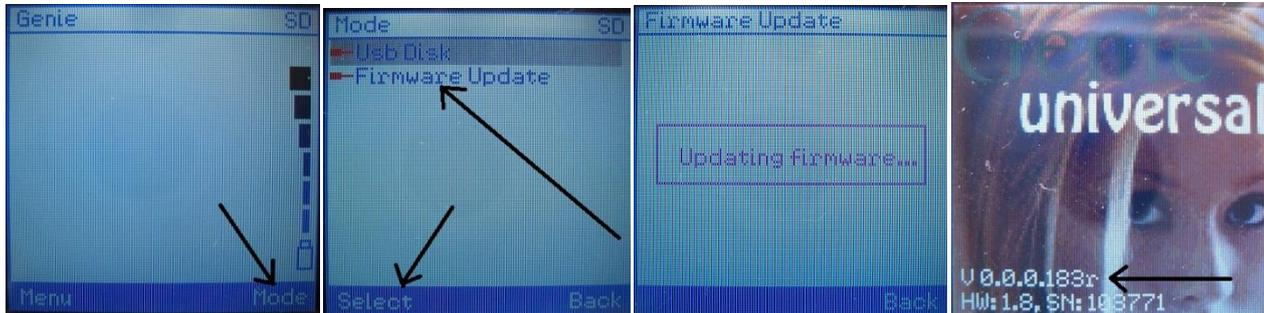
Genie-Universal will show on the LCD "Updating Firmware..." and will restart after 5-7 seconds with latest Firmware Inside.
