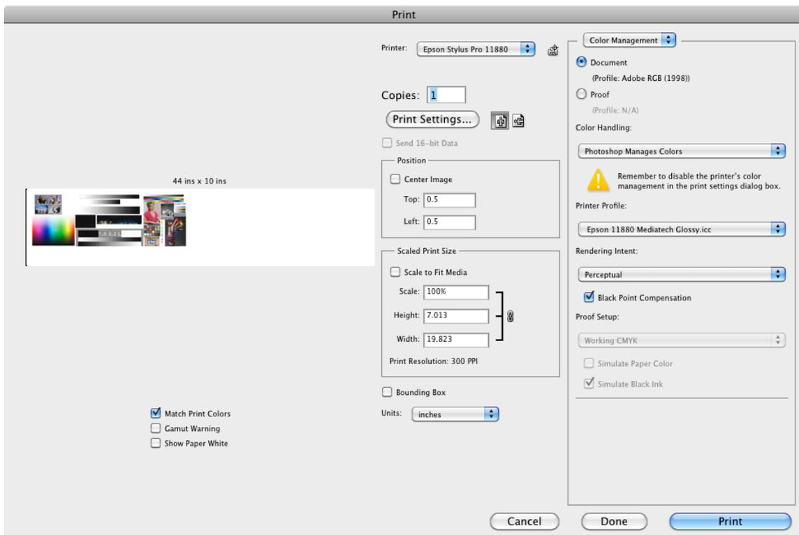
Make sure that “Epson Stylus Pro 11880” is selected as the printer. Don’t worry about page size, position, or scaling yet. This will be setup soon. First, set the colour handling:
