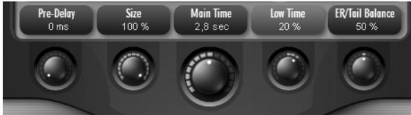
You can control up to five reverb parameters without even leaving the *Presets Page*: Knobs 1 to 3 have fixed assignments; knobs 4 and 5 may be configured at will.
