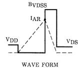
$\begin{array}{l} T_{ch}=25^{\circ}C \ (Initial) \\ Peak \ I_{AR}=5 \ A, \ R_{G}=25 \ \Omega \\ V_{DD}=16 \ V, \ L=1.0 \ mH \end{array} \\ \to AS=\frac{1}{2} \cdot L \cdot I^{2} \cdot ( \ \frac{BVDSS}{BVDSS-V_{DD}} )$
