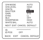
AUTO: Exposure time is controlled automatically within a range of 1/60 sec, to 1/100,000 sec to obtain an adequate signal.
