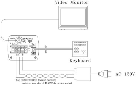
24V AC UL Listed Class 2 power suply / 12V DC power supply CAUTION: Never input 24V AC and 12V DC at the same time
