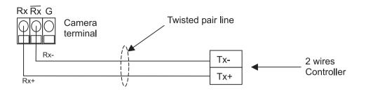
Tx of the communication line from KBD is connected to Rx of the camera, and Tx- is connected to Rx- of the camera.
