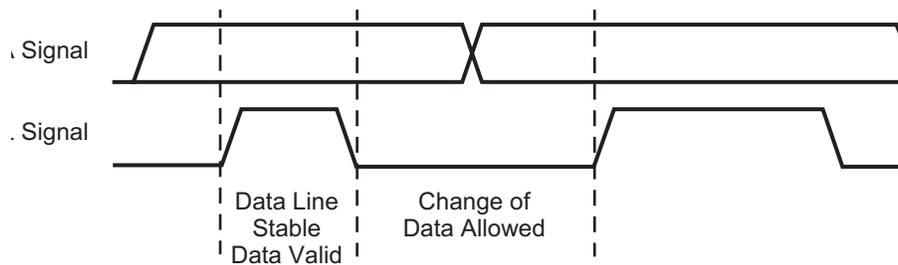
Figure 30. I<sup>2</sup>C Clock and Data Relationship
