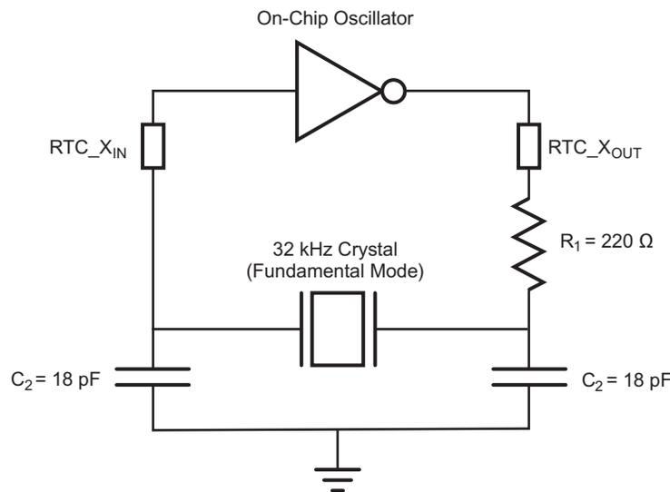
Figure 46. Recommended Crystal Oscillator Configuration (32KHz operation)
