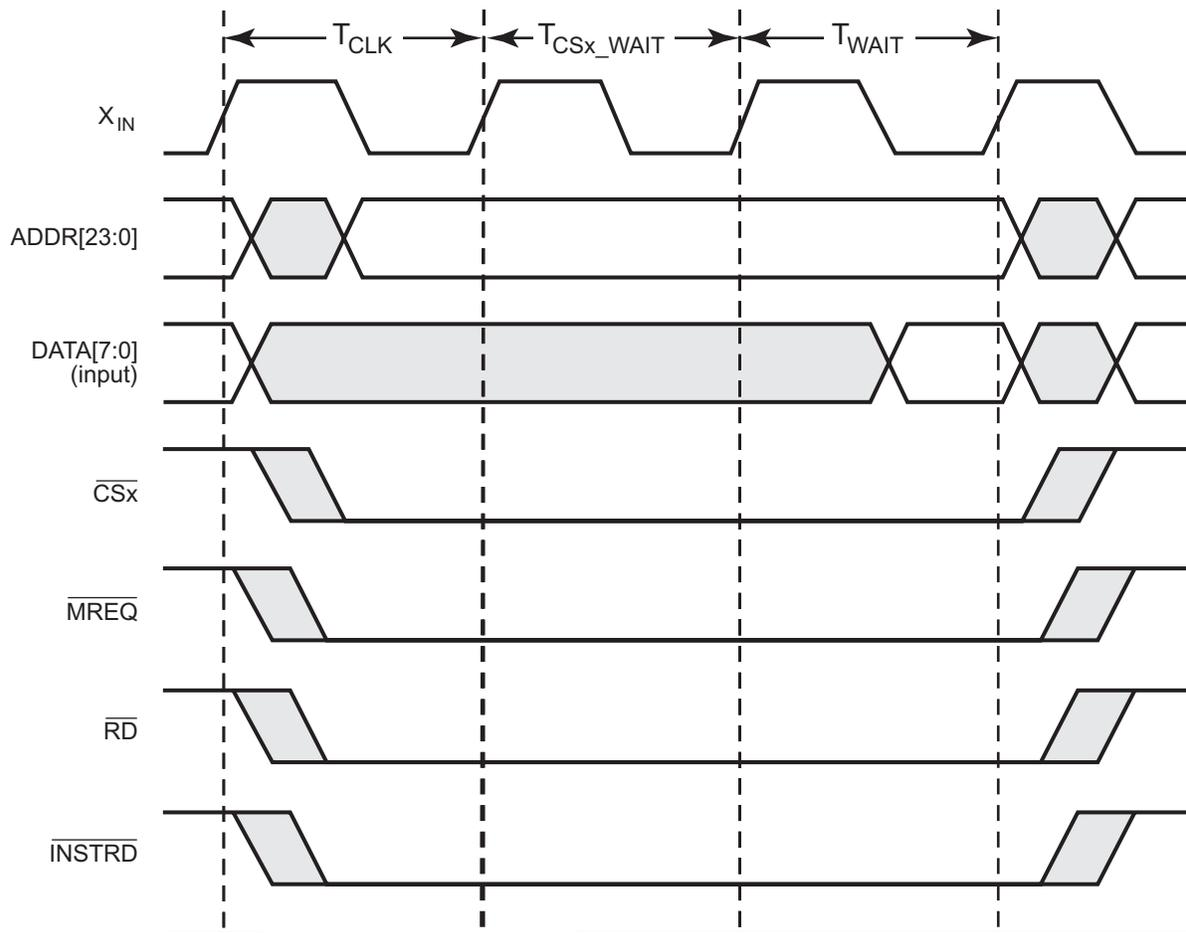
Figure 53. Wait State Timing for Read Operations
