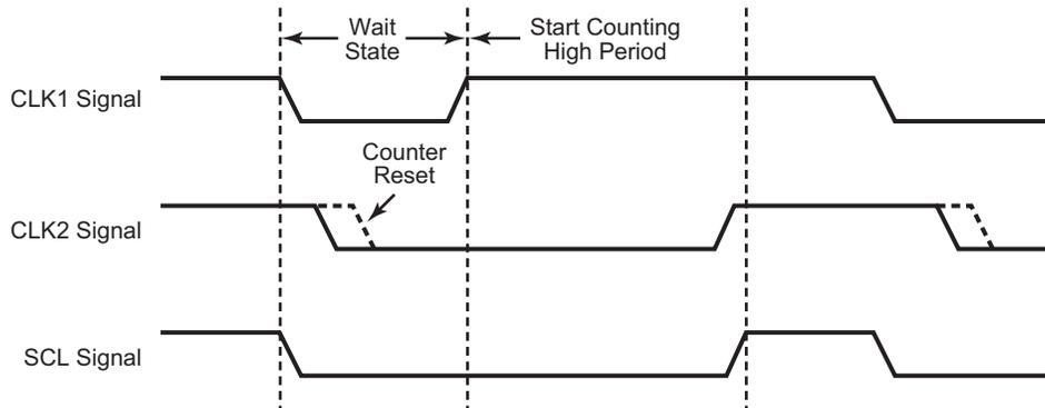
Figure 34. Clock Synchronization In I<sup>2</sup>C Protocol
