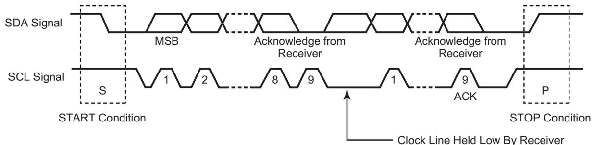
Figure 32. I<sup>2</sup>C Frame Structure
