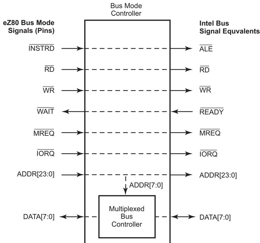
Figure 9. Intel™ Bus Mode Signal and Pin Mapping
