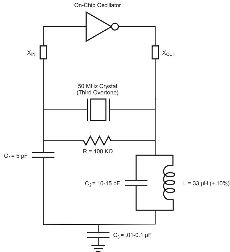
**Figure 45. Recommended Crystal Oscillator Configuration (50MHz operation)**
