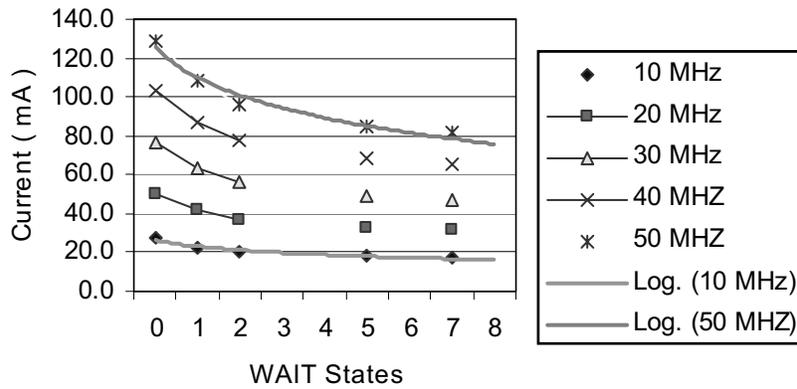
Figure 48. I<sub>CC</sub> vs. WAIT (Typical @ 3.3V, 25°C)
