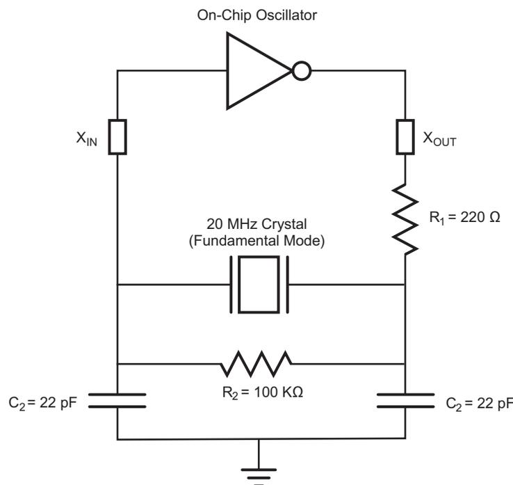
Figure 44. Recommended Crystal Oscillator Configuration (20MHz operation)
