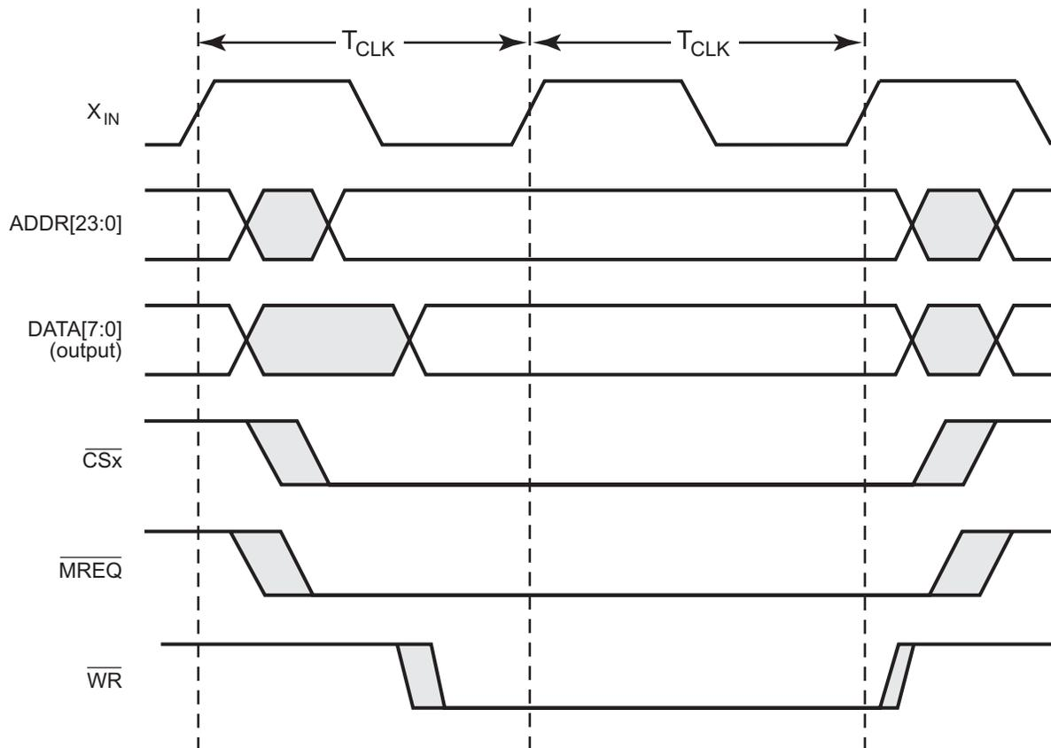
Figure 54. Wait State Timing for Write Operations
