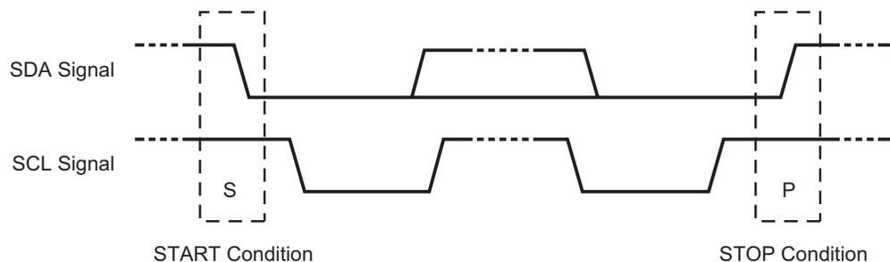
Figure 31. START and STOP Conditions In I<sup>2</sup>C Protocol
