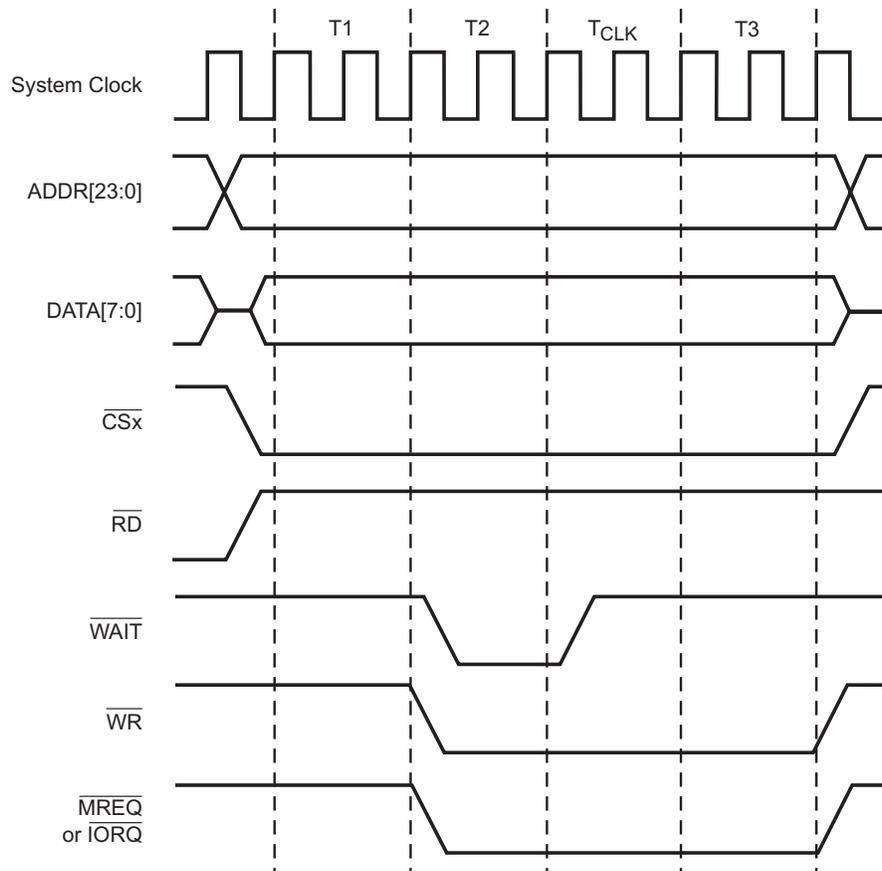
Figure 8. Z80 Bus Mode Write Timing Example
