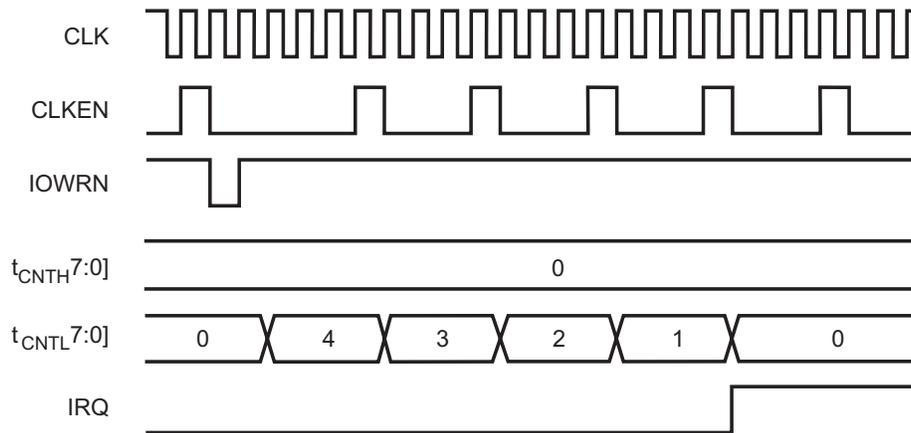
Figure 19. PRT Single Pass Mode Operation Example
