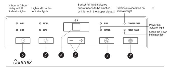
**NOTE:** When the bucket is full or removed, the controls cannot be set.
