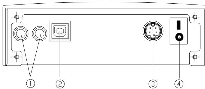
1. **音源输出接头 (Analog Audio Output Connector)**
