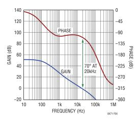
Figure 4. Bode Plot for Example Buck Converter
