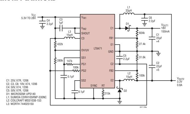
Figure 8a. Wide Input Range Buck Converter with 3.3V Output and Boost Converter with 18V Output at 400kHz
