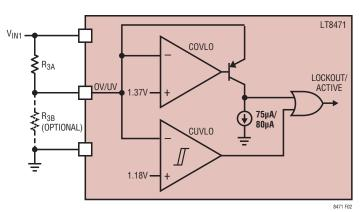
Figure 2. Configurable OVLO and UVLO
