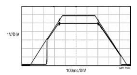
$\mbox{V}_{\mbox{\footnotesize CC}}$  (Yellow Trace) Is Ramped from OV Up to 6V and Then Back Down to OV. Channel 1 Output Voltage Is the Green Trace. It is Located by a  $5\Omega$  Resistor
