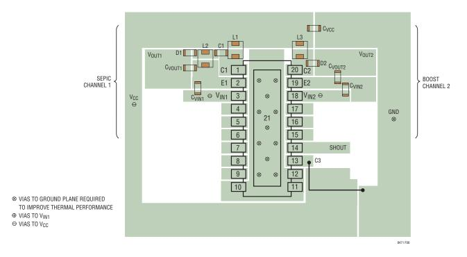
Figure 6. Suggested Component Placement for a SEPIC and Boost Converter
