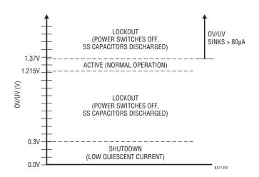
Figure 1. Chip States vs OV/UV Voltage
