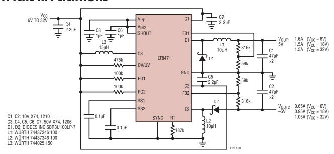
Figure 10a. Wide Input Range Converter with ±5V Output Voltages at 450kHz
