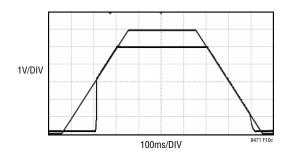
V<sub>CC</sub> (Yellow Trace) Is Ramped from OV Up to 6V and Then Back Down to OV. Channel 1 Output Voltage Is the Green Trace. It Is Located by a  $100\Omega$  Resistor
