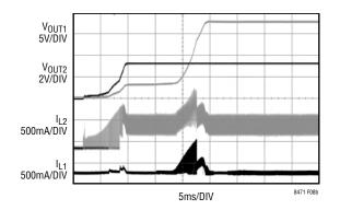
Figure 8b. Start-Up Waveforms
