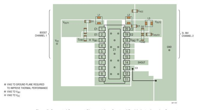
Figure 7. Suggested Component Placement for a Boost and Dual-Inductor Inverting Converter
