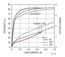
Figure 10b. Efficiency and Power Loss (Load from V<sub>OUT1</sub> to V<sub>OUT2</sub>)
