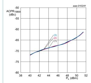
$V_{DS} = 28 \text{ V}; I_{Dq} = 3400 \text{ mA}.$
