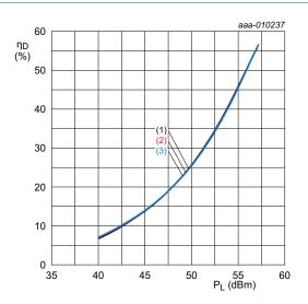
$V_{DS}$  = 28 V;  $I_{Dq}$  = 3400 mA;  $t_p$  = 100  $\mu s;$   $\delta$  = 10 %.
