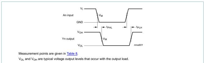
Fig 5. Propagation delay input (An) to output (Yn)
