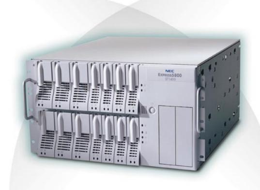
EC Computer Systems Division delivers the ST1400 Disk Expansion System, an external disk expansion unit that is designed to help you grow storage capacity beyond the internal limits of your server. With up to 14 hot-swap drive bays, redundant cooling fans, and hot-swap redundant power supplies, the NEC Express5800 ST1400
