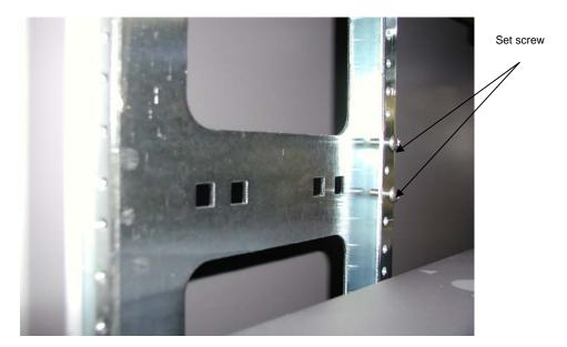
**40.** Hook each rail fitting the round hole in the rail onto the screws in step 1, and temporarily secure it.
