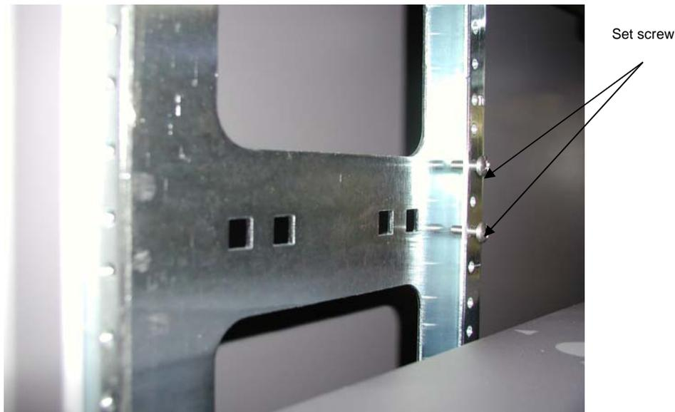
2. Hook each rail fitting the round hole in the rail onto the screws in step 1, and temporarily secure it.
