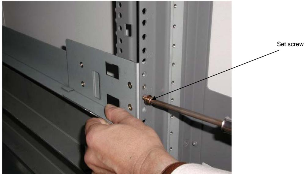
6. Next, secure the fixture, where the cable tie has been passed through, to the rack by screwing the set screw (M5 screw) into the upper female threaded hole.
