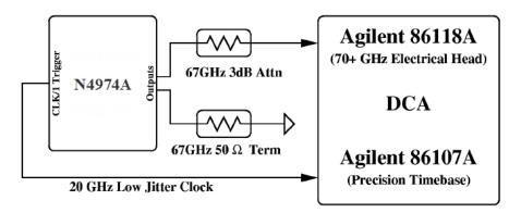
Figure 5. Verification setup
