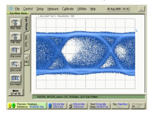
Figure 12. Eye with re-timer out of phase alignment
