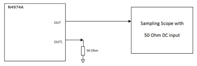
Figure 10. Termination using direct connection to a DC-coupled 50 ohm scope input
