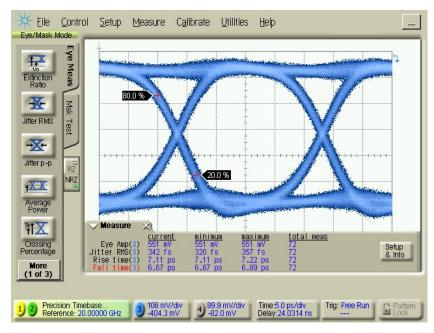
Figure 6. 40 Gb/s eye output from N4974A
