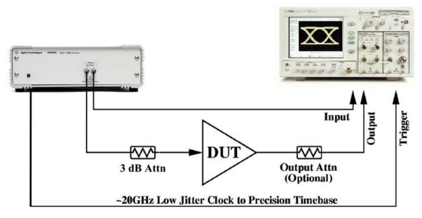
Figure 7. N4974A generic test example experimental setup
