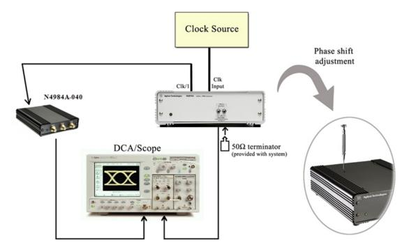
Figure 11. Re-timer phase adjustment setup
