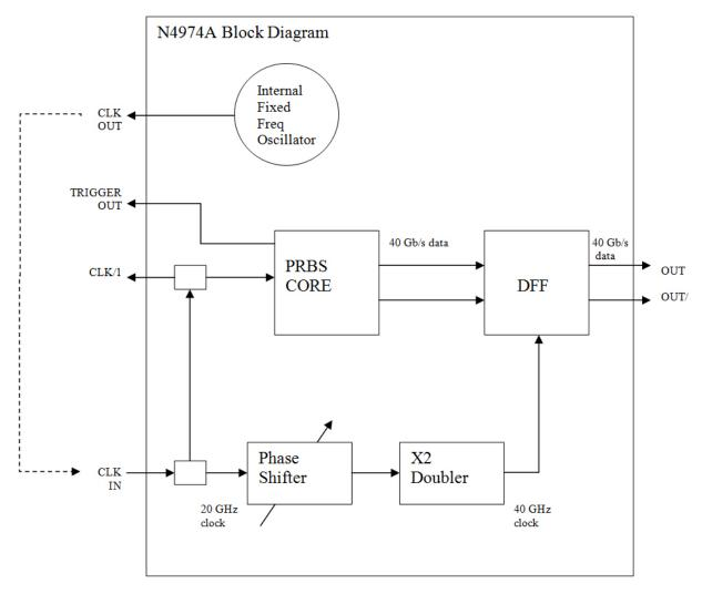
Figure 4. N4974A block diagram
