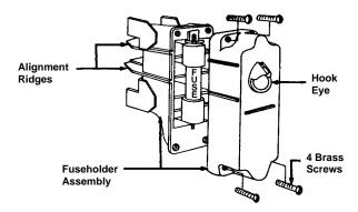
DANGER: DO NOT ATTEMPT TO REPLACE FUSES WITHOUT FIRST WITHDRAWING THE FUSEHOLDER ASSEMBLY FROM THE HOUSING. FAILURE TO DO SO WILL RESULT IN SEVERE INJURY, DEATH OR PROPERTY DAMAGE.
