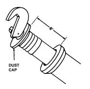
JERK THE FUSEHOLDER OUT APPROXIMATELY 6" TO OPEN THE CIRCUIT. WAIT A FEW SECONDS FOR OIL TO DRAIN BACK INTO THE TANK, THEN COMPLETELY WITHDRAW FUSEHOLDER.
