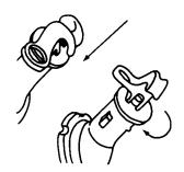
PUSH DOWN AND ROTATE THE HANDLE 90° CLOCKWISE IN THE HOUSING TO BREAK ANY ADHESION BETWEEN THE GASKET AND THE HOUSING.
