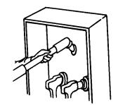
ATTACH HOT-LINE TOOL TO HANDLE EYE, STAND TO ONE SIDE AND UNLOCK THE HANDLE.
