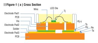
electrode of the outer shell to solder. The thermal resistance between the junction section of the light-emitting diode and the electrode side of the outer shell is Rj-s and the specific thermal resistance value of the package. Therefore, the following formula is used:
