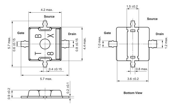
79A Package Recommended P.C.B. Layout (Unit: mm)
