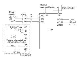
Figure 3.20 Connecting a Braking Resistor
