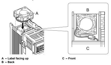
Figure 6.2 Cooling Fan Orientation
