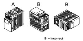
Figure 2.1 Correct Installation Orientation
