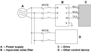
Figure 7.7 Input-Side Noise Filter (Three-Phase 200/400 V)
