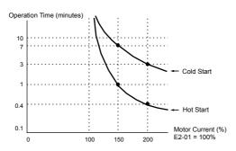
Figure 4.19 Motor Protection Operation
