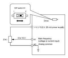
Figure 4.7 Voltage Input for the Frequency Reference
