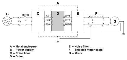
Figure 7.10 Reducing Radio Frequency Noise
