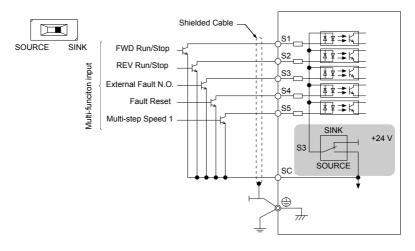
Figure 3.17 Sinking Mode: Sequence from NPN Transistor (0 V Common)
