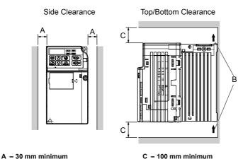
Figure 2.2 Correct Installation Spacing
