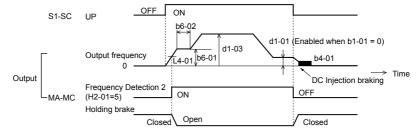
Figure 4.21 Holding Brake Time Chart
