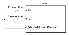
Figure 4.9 Example Wiring Diagram for 2-Wire Sequence
