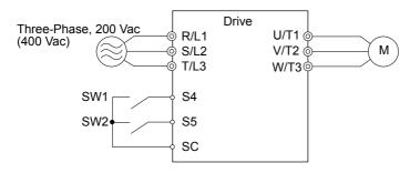
Figure 4.14 Control Terminals for 4 Multi-Step Speeds
