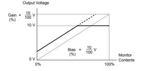
Figure 4.18 Analog Output Gain/Bias Setting
