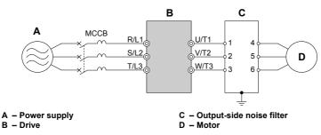
Figure 7.8 Output-Side Noise Filter
