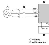
Figure 7.5 Connecting a DC Reactor
