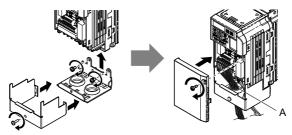
A - Pass power wiring and control signal wiring through different exit holes at the bottom of the drive.
