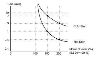
Figure C.8 Motor Overload Protection Time
