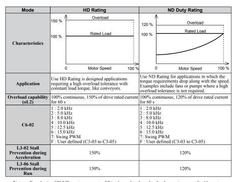
By selecting HD/ND, motor parameter E2 is changed to the value for the maximum applicable motor. Note:
