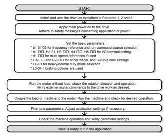
Figure 4.6 Basic Start-Up and Motor Tuning
