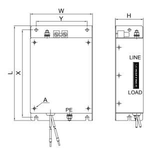
Figure C.6 EMC Filter Dimensions
