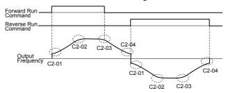
Figure 4.13 S-Curve Characteristics
