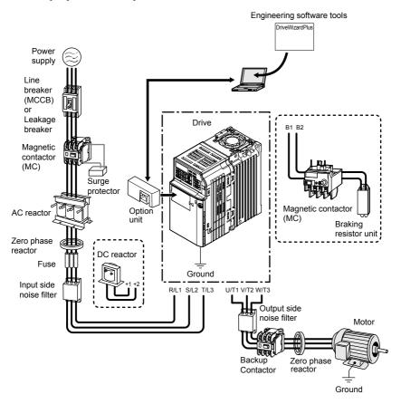
Figure 7.1 Connecting Peripheral Devices
