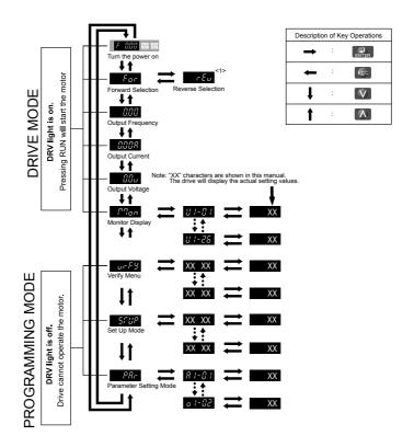
Figure 4.3 Digital LED Operator Screen Structure
