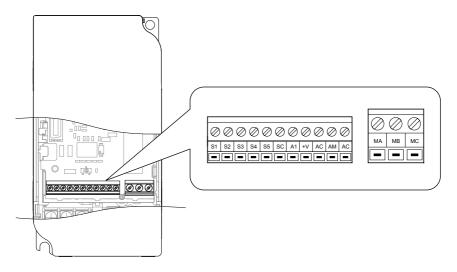
Figure 3.11 Control Circuit Terminal
