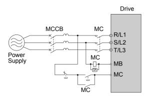
Figure 7.2 Connecting a MCCB (Three-Phase 200 V Class)
