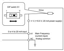
Figure 4.8 Current Input for the Frequency Reference
