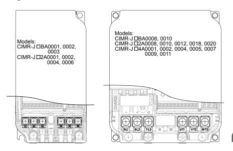
Figure 3.5 Main Circuit Terminal Block Configurations
