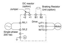
Figure 3.3 Connecting Single-Phase Main Circuit Terminals
