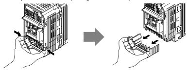
Figure 3.7 Remove the Terminal Cover on an IP20/Open-Chassis Drive
