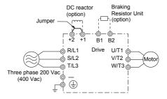
Figure 3.4 Connecting Three-Phase Main Circuit Terminals
