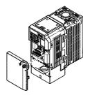
Figure 7.12 Remove the Front Cover on a NEMA Type 1 Drive
