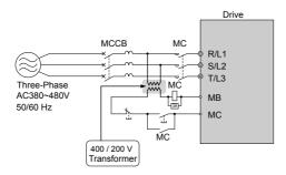
Figure 7.3 Connecting a MCCB (Three-Phase 400 V Class)
