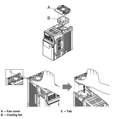
Figure 6.1 Remove the Cooling Fan Cover
