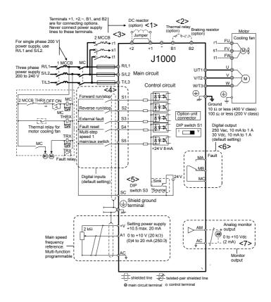
Figure 3.1 Drive Standard Connection Diagram (200 V Class Example)
