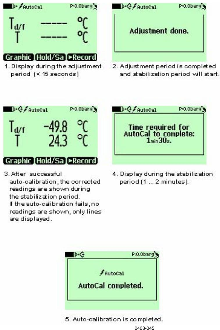
**Figure 9** Auto-Calibration Displays
