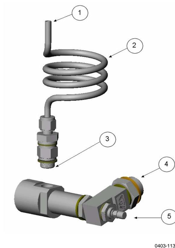
**Figure 23** Alternative Assembly of DSC74C for Tight Spaces
