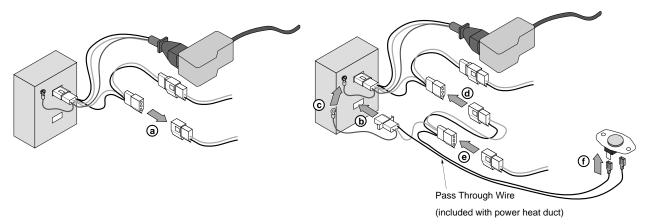
(g) Attach the romex from the rheostat to the fireplace circuit following the directions below.
