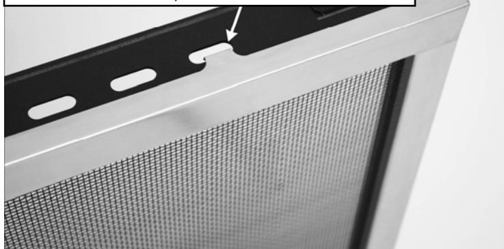
G. Apply the upper and lower horizontal trim sections so the hooked edge of the tabs fits into a slot in the sides of the glass frame. The ends of the horizontal trim sections cover and align with the ends of the vertical trim sections. See Photo 3.
