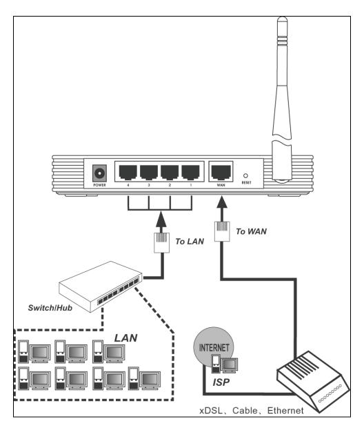
Figure 2-1 Hardware Installation of the TL-WR541G 54Mbps Wireless Router
