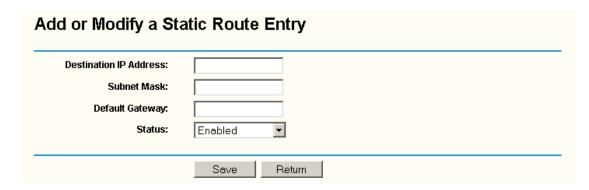
Figure 4-50 Add or Modify a Static Route Entry
