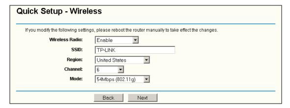
Figure 3-9 Quick Setup - Wireless settings
