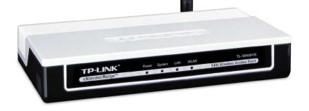
Adopts eXtended Range™ technology, 4-9 times the signal coverage of traditional 11b/g products Supports multiple operating modes (Access Point, Client, Universal/ WDS Repeater, Wireless Bridge)
