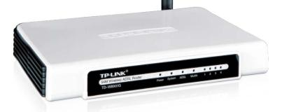
3-in-1: ADSL2+ modem, 4-port Ethernet router and wireless G access point Latest ADSL standards for superior performance: up to 24Mbps downstream and 3.5Mbps upstream
