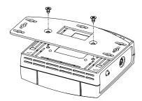
Mounting TOY-SC1 with SIRIUS SCC1 Bracket Assembly
