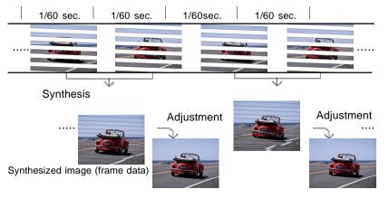
If the subject is moving, however, the data for the two fields is slightly different, and it is not possible to achieve a clear still image simply by synthesizing the fields. "Image adjustment" refers to digital processing of the data to achieve a clear still image. PixLab offers a choice of two types of Image adjustment.
