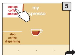
To brew an amount of coffee greater than that preset by the manufacturer, press "custom coffee amount" before the end of the brew cycle in progress. When the quantity is reached, press "stop coffee dispensing".
