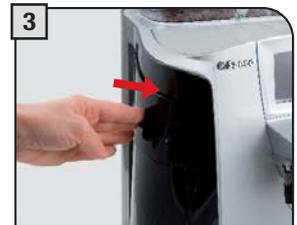
3 Close the container and put it back in its appropriate seat. Make sure to carefully close the compartment.
