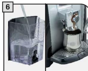
Put a container under the water spout. When the water tank is inserted the machine automatically proceeds to prime the water circuit. If this operation is not successful, consult "manually priming the circuit" (see page 6)
