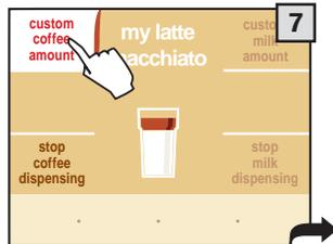
The brew cycle may be interrupted only by pressing "stop coffee dispensing". If the button is not pressed, the coffee may overflow.
