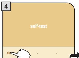
If desired, the "demo" function (see page 28) may be activated by pressing the key, each time the machine carries out a self-diagnosis.
