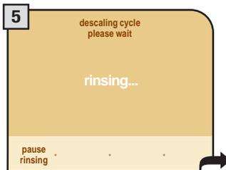
The machine performs the rinse cycle. At the end of the rinse cycle fill the tank with fresh drinking water. Before filling the tank reinsert, if desired, the water filter again, or reinsert the small white filter (see page 7).
