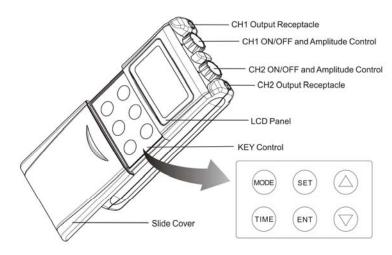
Your device offers two controllable output channels. This device creates electrical impulses whose amplitude, duration, and modulation can be altered with the controls or buttons. The device controls are very easy to use and the slide cover protects accidental changes in settings.
