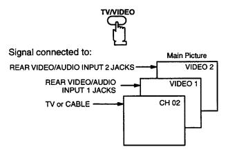
Signal connected to:
