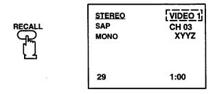
**R–Tune (Rapid Tune) Button** – Press the R–TUNE (RAPID TUNE) button to instantly switch between the last two channels selected (without any On Screen display being activated).
