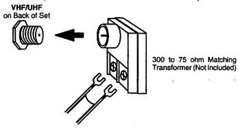
**Cable Connection** – For reception of cable channels (01~125) connect the cable supplied by your local Cable company. Antenna Mode must be set to CABLE. (Refer to Antenna Mode section.)
