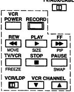
**TV/Video Button** – Press the TV/VIDEO button to select desired input for Main Picture or PIP frame (when PIP frame is displayed).
