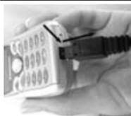
When charging is completed, disconnect the charger from the AC wall outlet. Grasp the Fast Travel Charger connector and push downward to release it from the base of the phone.
