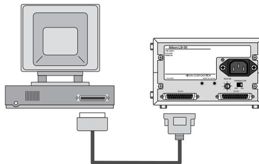
If there are other external devices in the chain, connect the scanner to the last of these devices.
