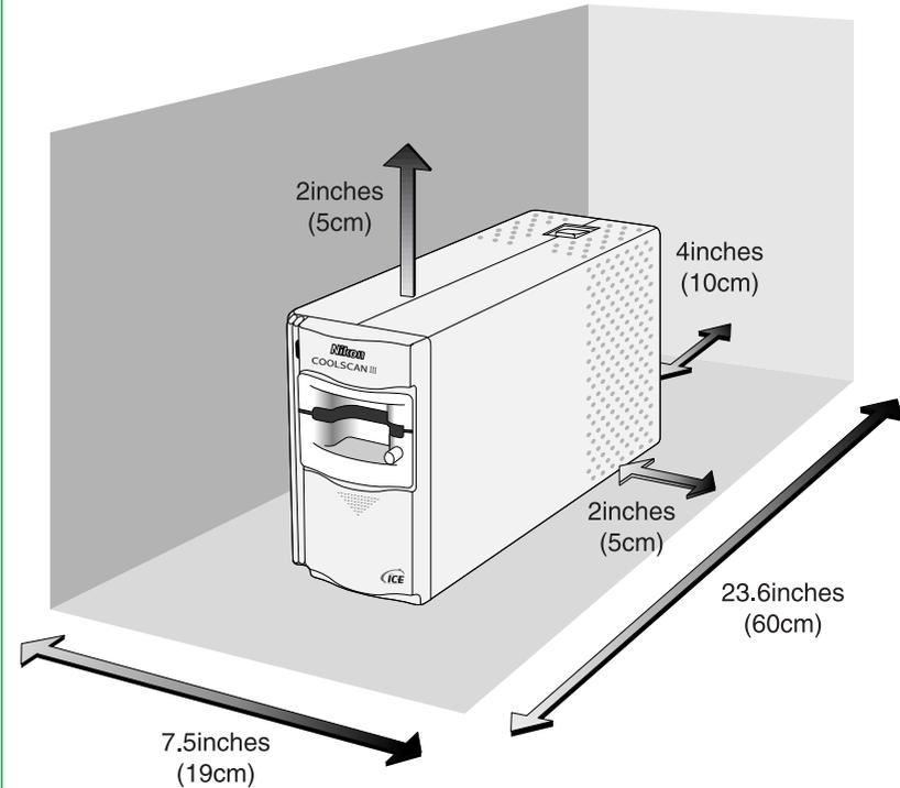
**✓ Caution:** The scanner must be installed with its feet down, as shown in the illustrations on this page. Do not store or operate the scanner in any other orientation.
