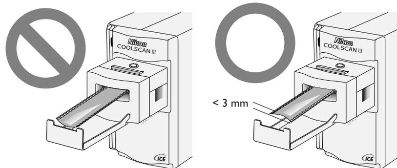
Film will be ejected from the scanner automatically when the scanner is turned on or when no operation is performed for several minutes. Film can also be ejected using the software provided with your scanner. For details of scanning operations, refer to the **User's Guide** or software reference manual.
