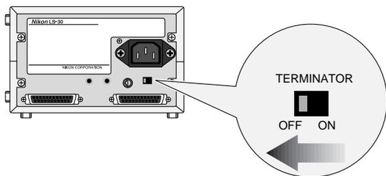
Connect one end of the SCSI cable to either of the connectors on the rear of the scanner, then connect the other end to one of the devices in the chain.
