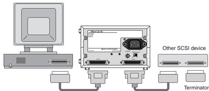
**Note:** If the last device in the chain has an unused SCSI connector, a separate terminator should be attached to it, even if the device is connected to the SCSI chain using a through terminator.
