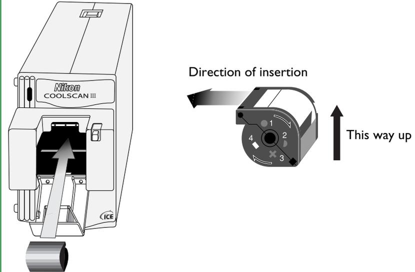
Close the cover, pushing it closed until the latch snaps into place. The scanner will automatically feed film from the IX240 cartridge into the scanner. For details on scanning IX240 film, see the software reference manual.
