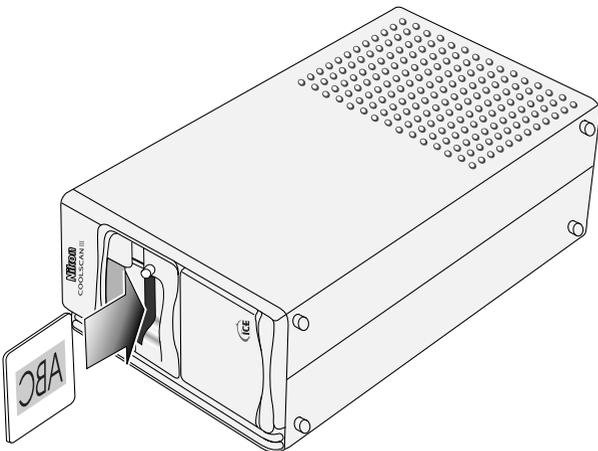
The correct orientations for inserting landscape and portrait slides are shown below. If the slides are inserted with the top and bottom of the image reversed, this can be corrected after scanning using the software provided with your scanner.
