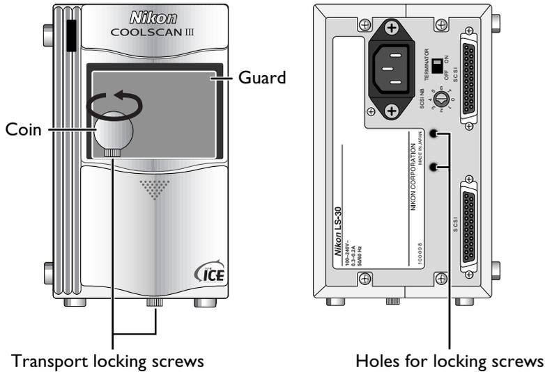
**Caution:** Never turn the scanner on with the locking screws in place. Turning the power on in these circumstances could damage the scanner.
