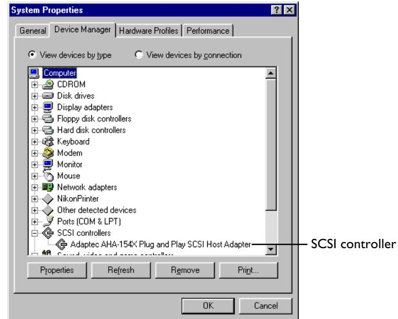
2. If the card has been installed correctly, the System Properties window will contain a "SCSI controllers" icon. If a "?", "!", or "X" is showing next to the name of the SCSI adapter, there is a problem which must be resolved before the scanner can be connected. To determine the cause of the problem, select the adapter icon and click the **Properties** button to view the drivers and system resources for the device.
