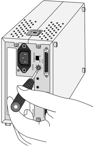
**Note:** The LS-30 conforms to Level 1 of the SCAM (SCSI Configuration Auto-Magically) SCSI-selection standard, which allows some computers to set the scanner's ID automatically. If your computer's operating system supports Plug&Play and the SCSI host (computer or SCSI extension board) conforms to SCAM, the scanner may be automatically assigned an ID which differs from that set using the SCSI ID dial. SCAM will not assign conflicting IDs to SCSI devices.
