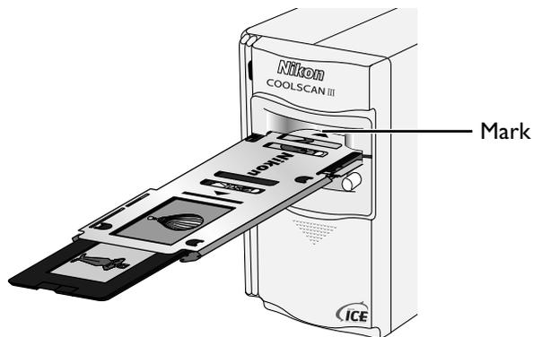
When removing the holder from the adapter, wait until the status LED glows steadily, then slide the holder out by hand. Do not use the eject button.
