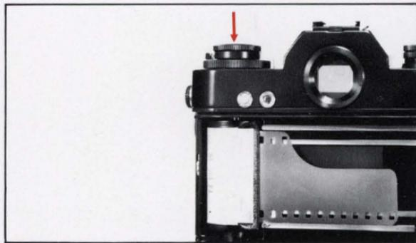
knob and turn it gently in the direction of the arrow until you feel a slight resistance. This takes up any slack in the film cartridge. Then fold back the rewind crank.
