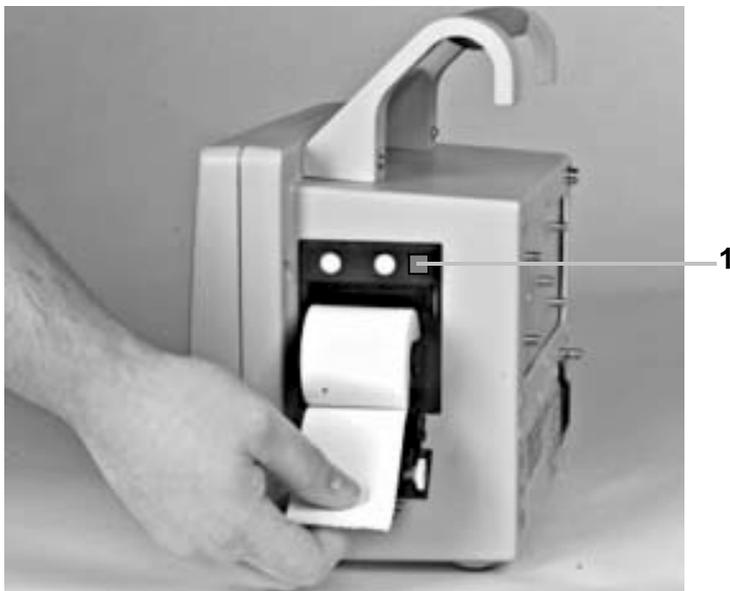
**Figure 29: Loading Thermal Paper in Printer**
