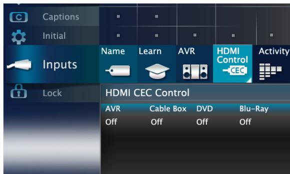
Select **On** or **Off** to enable or disable the TV's control of a CEC-enabled device. See the TV owner's guide for use of this feature.
