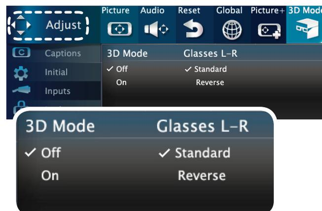
Use the **Adjust > 3D Mode** menu to enable 3D video viewing.
