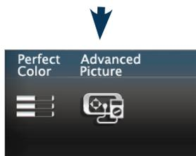
**PerfectColor** Sliders adjust the saturation (intensity) of six colors for the current input.
