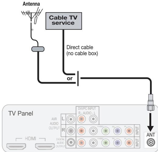
Mitsubishi recommends using coaxial antenna cable instead of flat twin lead antenna wires for better performance.
