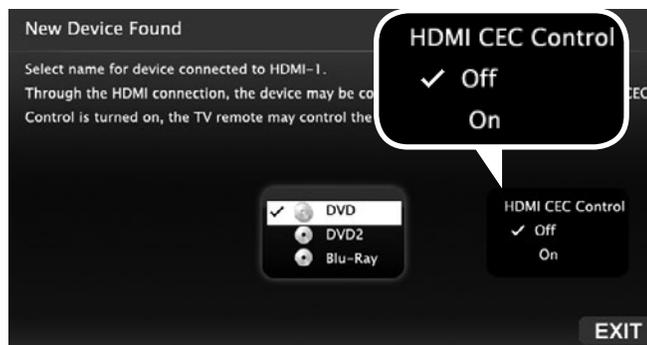
*New Device Found* screen for a device with HDMI control enabled. Select **On** if you want to enable the TV's HDMI control of the device. In some cases, as in the example, you will also be prompted to select a device name.
