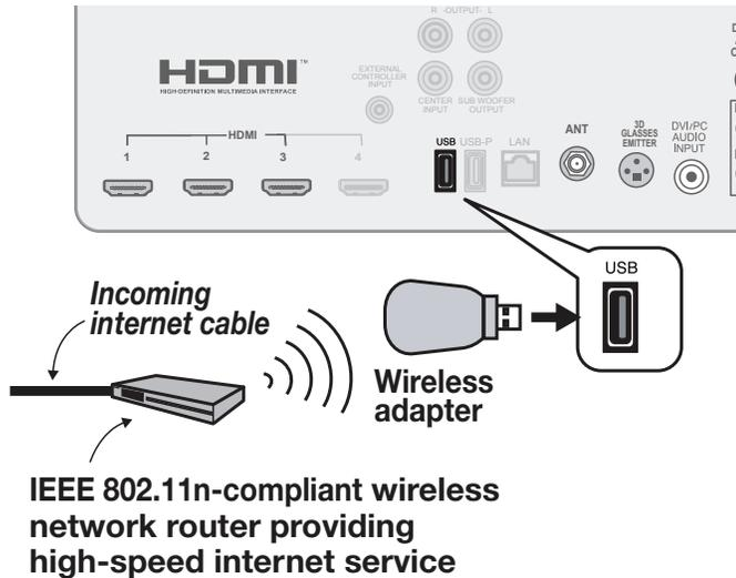
Connect the USB adapter to the USB port on the back of the TV. **840 Series.** Use the left USB port.
