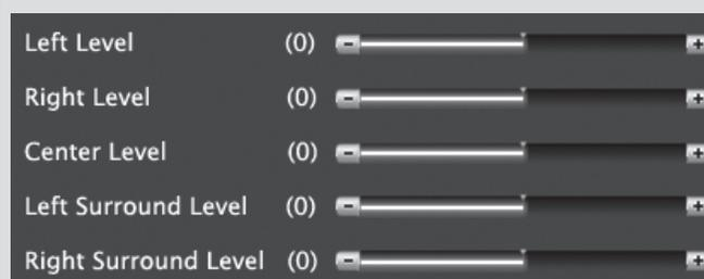
Adjust the volume level of individual audio beams using sliders in the SoundPro > Custom menu.
