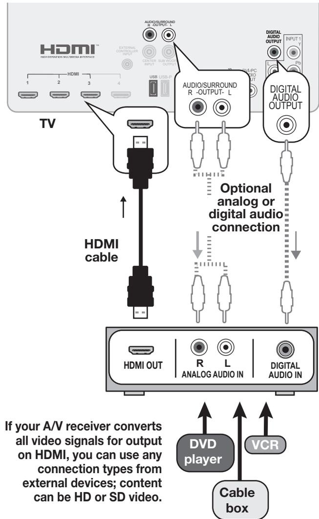
If your A/V receiver converts all video signals for output on HDMI, you can use any connection types from external devices; content can be HD or SD video.
