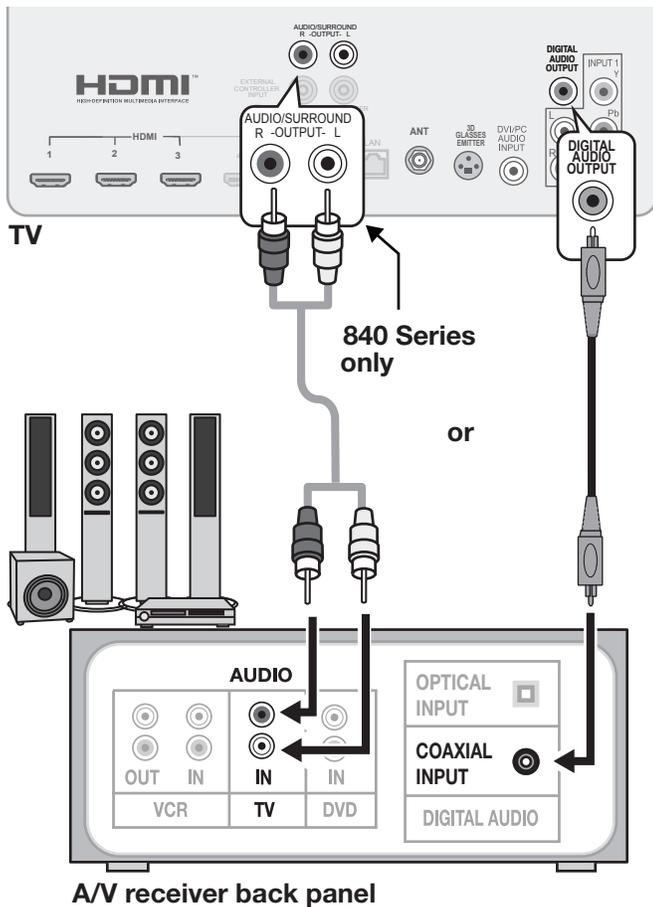
**Note:** On rare occasions, an HDMI signal may be copy-restricted and cannot be output from the TV as a digital signal. To hear these copy-protected signals through the A/V receiver, use the connection for an analog A/V receiver.
