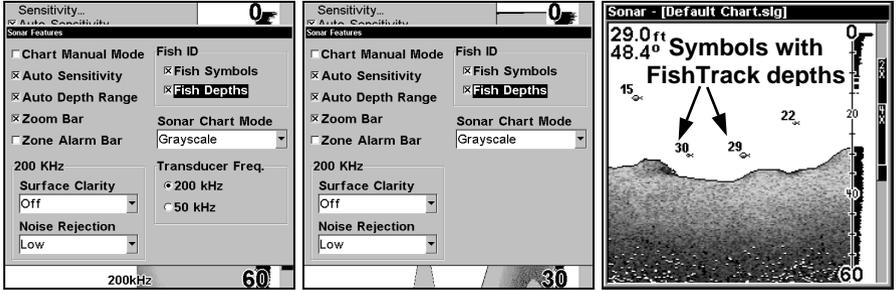
Sonar Features menu with Fish I.D. Depths selected (Left, dual-frequency menu; center, single-frequency menu). When the check box to the left is checked, the feature is on. Right, Sonar Page showing Fish I.D. symbols and FishTrack depths turned on.
