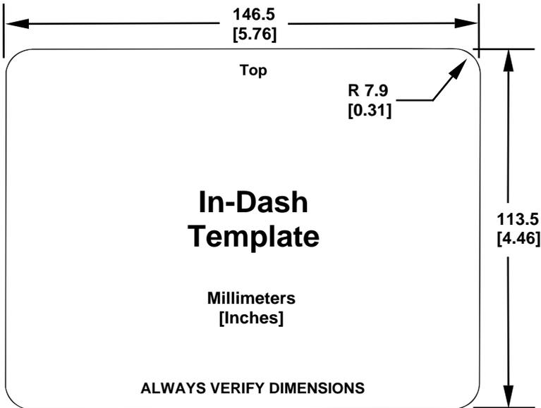
**In-dash mounting template for the sonar unit, showing dimensions. NOTE: The figure above is *not* printed to scale. A scaled template (FM-5 In-Dash Adapter Kit instructions) is available for free download from our web site, [www.lowrance.com](http://www.lowrance.com).**
