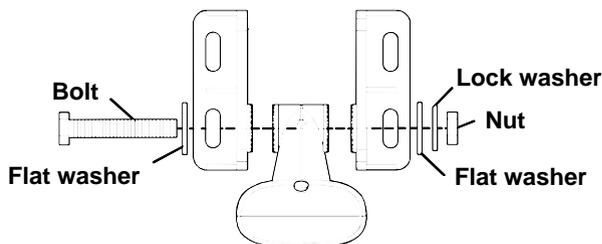
Assemble transducer and bracket.
