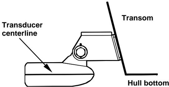
**Align transducer centerline with hull bottom.**
