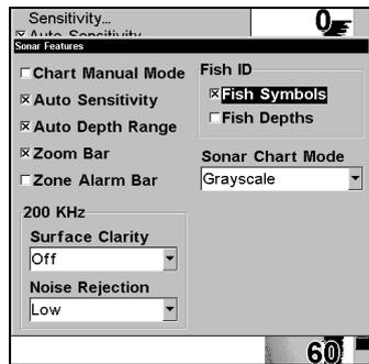
Sonar Features menu with Fish I.D. Symbols selected (Left, dual-frequency menu; right, single-frequency menu). When the check box to the left is checked, the feature is on.
