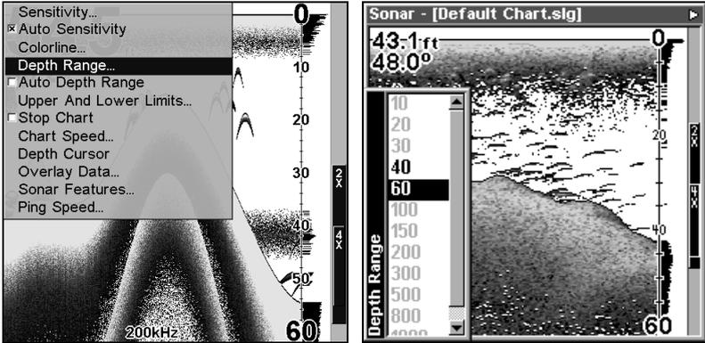
Left, Sonar Page menu with Depth Range command selected. Right, the Depth Range Control Scale.
