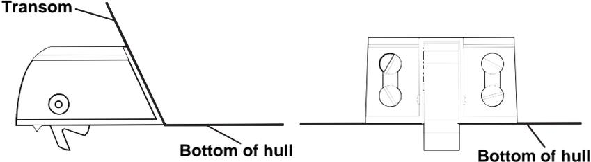
Speed sensor mounting configuration:
