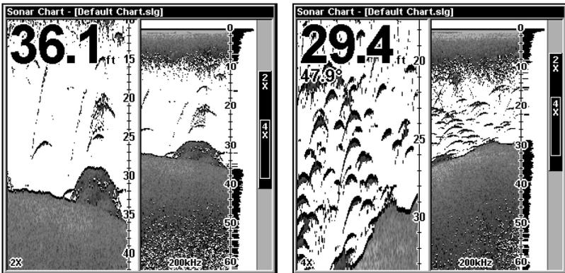
**Split Zoom Sonar Chart.** Left, image shows the left window zoomed to 2X. The image on the right shows the left window zoomed to 4X. The depth overlay data is set to the default large text size; the water temperature is set to the small text size.
