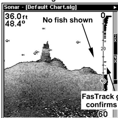
Left, figures 1A and 2A show Sonar Page in normal chart mode. Right, figures 1B and 2B show the same underwater scene with Fish I.D. turned on. Note how arches are replaced with symbols.
