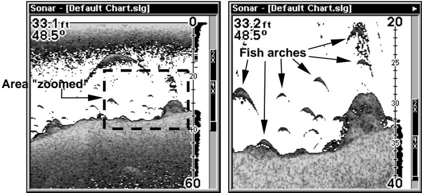
Normal display, in auto depth range mode, left. Right, display "zoomed" with Upper and Lower Limits focusing on the portion of the water column from 20 feet to 40 feet deep. In the "zoomed" image, note the target definition at lower left, showing a fish holding just above the structure. Top right, two game fish are attacking a school of bait fish.
