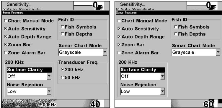
Sonar Features menu with Surface Clarity selected (Left, dual-frequency menu; right, single-frequency menu).
