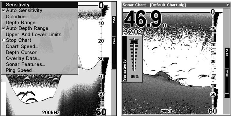
Left, Sonar Menu with Sensitivity command selected. Right, the Sensitivity Control Bar.
