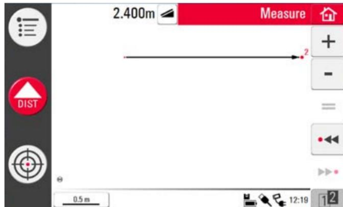
6. After the third point is measured a proposed "closing line" appears between the first and last measured point. The selected line is always highlighted with a bold line and an arrow in the direction of measurement.
