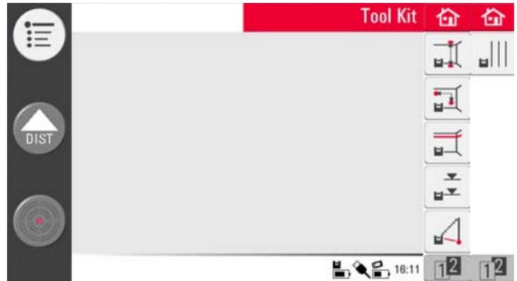
The Tool Kit applications offer quick, precise and easy-to-use tools for plumbing, metre marks, heights, and parallels. After each layout task the respective tool has to be restarted. A pop-up offers to continue with the same reference or to measure a new one. Data is not stored and cannot be imported or exported. Remote Control functionality is not supported in these applications.
