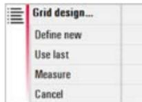
2. For a **new grid** pop-up prompts to enter column and row spacing and then to choose if horizontal or vertical shift of row or column is needed.
