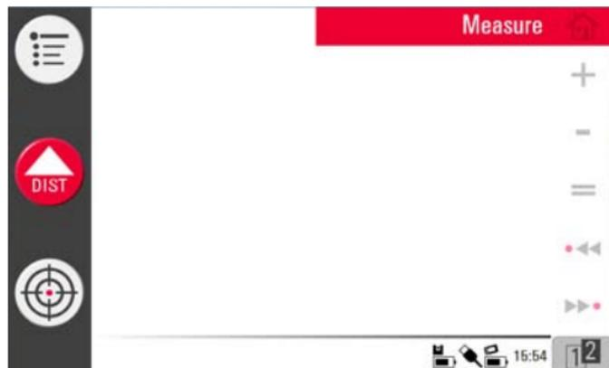
3. To target the first point, for example a corner, press
