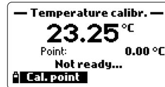
**NOTE** The meter allows a maximum difference of  $\pm 2^{\circ}\text{C}$  between the current reading and the set value. If this condition is not satisfied, the display will show the message “Max +/-2°C is allowed”.
