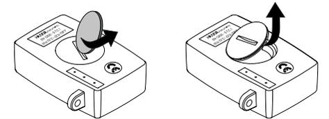
Insert the new battery with the + sign facing up, tight back the compartment cover and program the instrument.
