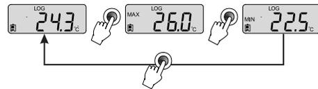
If you keep the button pressed, after 2 seconds the display will show alternatively (toggle every 2 seconds) the high and low alarm thresholds.
