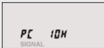
Figure 4. 10 Base-T signal detected, wired to PC.
