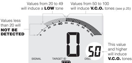
This discrimination interface for the Gold Bug DP was designed especially for relic-hunting. Relic hunters want control over what sizes of iron are detected, and also control over which targets are detected with a low-tone. Target values of 40 or less are ferrous.
