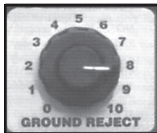
Figure 9. The GROUND REJECT control consists of a coarse-adjustment knob on top of a fine-adjustment knob.
