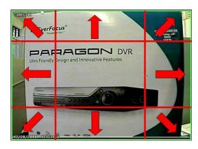
clicking the mouse when the directional arrow is displayed will move the viewing window one step in the direction of the arrow. Upon exiting the zoom function, the screen will return to the display as it was before entering the zoom function.
