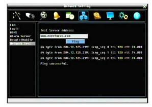
DNS functionality can also be confirmed by entering a valid DNS name instead of an IP address.
