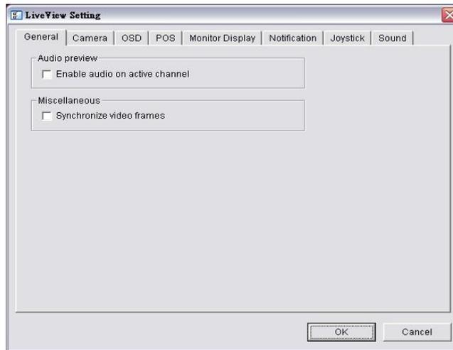
5. Check the **Enable audio on active channel** option to enable audio streaming on active channel. This function synchronizes with right click on camera to enable audio.
