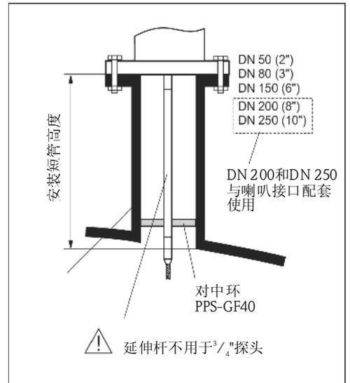
**在DN200/8"和DN250/10"的安装短管内安装**
