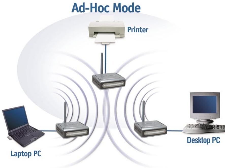
This example illustrates an **Ad-Hoc** setup. Simply connect the DWL-G810 (*refer to the Quick Installation Guide*) to your Ethernet-capable network device and you will be able to connect wirelessly with other devices also connected to DWL-G810's.
