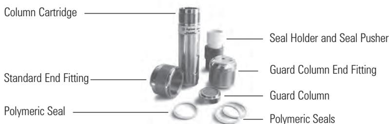
PrepHT cartridge columns have a unique design that makes them easy to install and seal finger-tight up to 5000 psi. The cartridge design allows for an integral guard column to be used, which prolongs the life of the purification column. This cartridge configuration is economical to use since the column cartridge and/or the guard cartridges are replaced independently. The end fittings are used many times.
