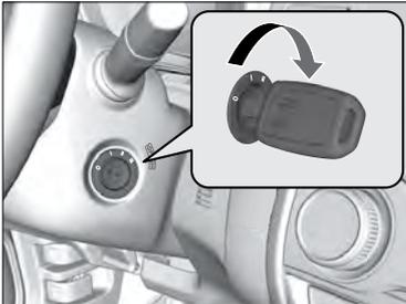
3. Coloque o interruptor da ignição na posição **LIGADO**
