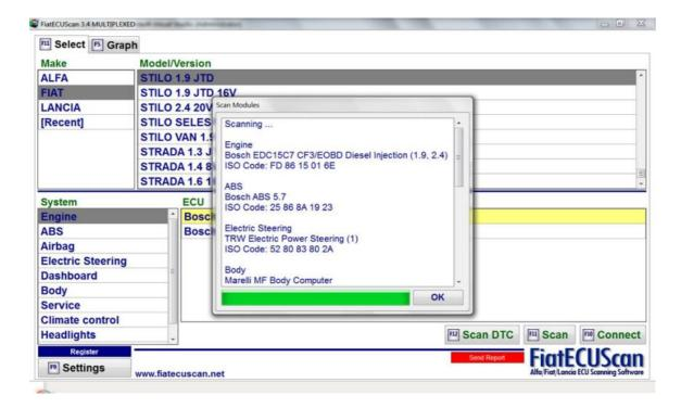
7. Click this button (or press F12 on your keyboard) to scan your vehicle for supported control modules and check each module for errors. This function works the same way as the "SCAN" function but it also checks each of the discovered modules for errors and shows the error codes.
