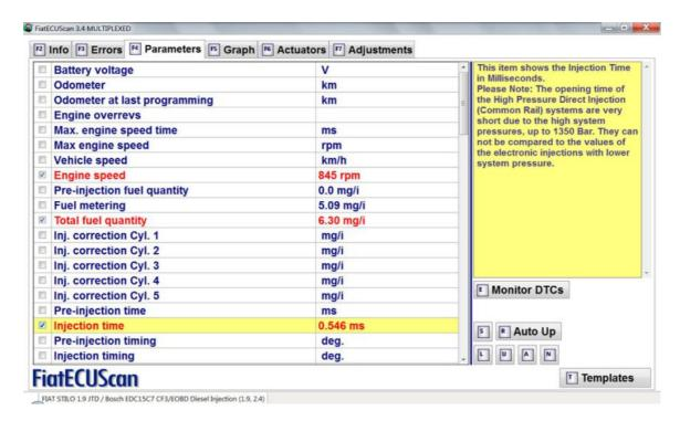
Here we selected 3 parameters – Engine speed, Total fuel quantity and Injection time
