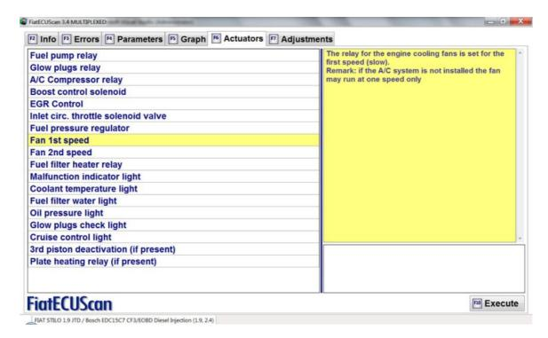
We see all tests which are available for this control module. We will select "Fan 1<sup>st</sup> speed" and execute it.
