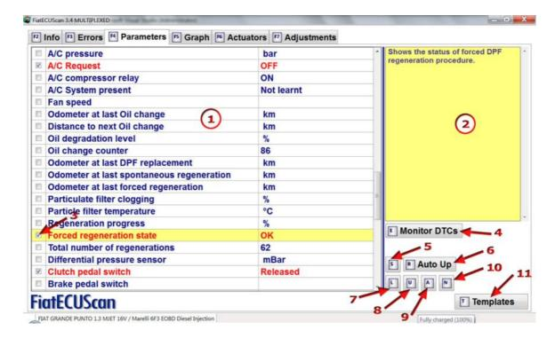
1. On this section of the screen are listed all available parameters for the module. You can go up/down the list using up/down arrow keys on your keyboard or using the mouse.
