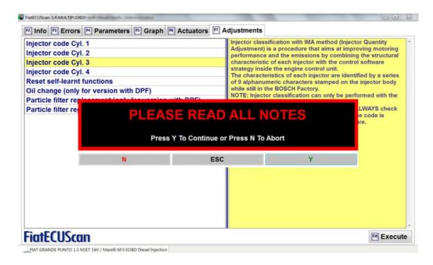
**Step 7:** We confirm that we have read the notes by pressing Y. Then the system will show a data entry window with current IMA code (obtained from the engine control module).
