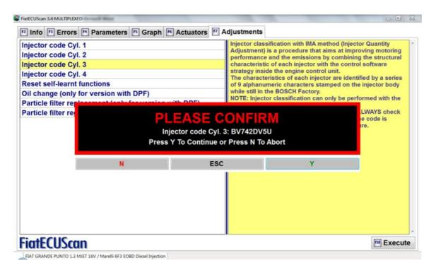
After you press Y the system will start writing the new code to the engine control module.
