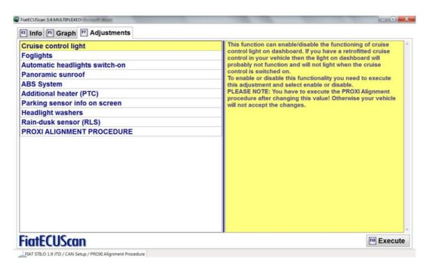
**Step 5:** Select "Cruise control light" and press F10 to execute this adjustment. The system will show current value of the setting.
