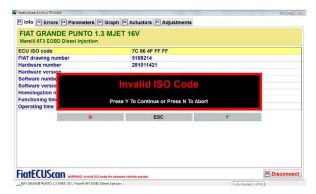
The "Invalid ISO Code" message means that the ISO code obtained from the vehicle is not recognized by FiatECUScan as correct for selected control module. In most cases this simply means that you have selected incorrect control module from FiatECUScan main screen. So, that you simply have to disconnect, then select different control module from FiatECUScan main screen and try to connect again.
