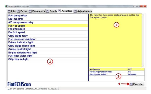
1. On this section of the screen are listed all available actuator tests for the module. Here you can select which test you want to execute.
