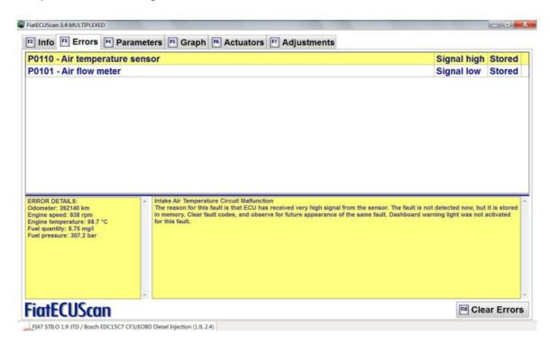
As you can see this control module reports 2 errors. Actually, I intentionally created these 2 errors by unplugging the MAF connector while the engine was working.
