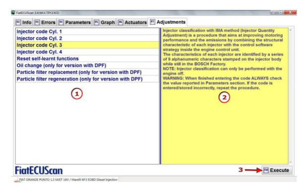
1. On this section of the screen are listed all available calibration/configuration procedures for the module. Here you can select which procedure you want to execute
