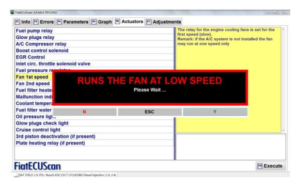
We press F10 and FiatECUScan will start executing this test. The engine cooling fan starts to work at low speed for a few seconds.
