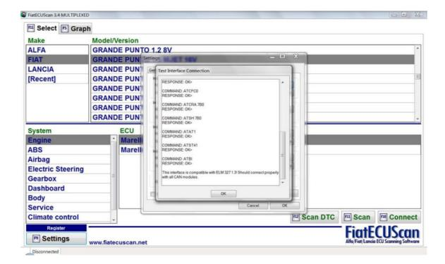
The result of all commands should be OK. If any of the commands has a different result then most probably the software inside the ELM interface is not compatible with ELM 1.3.
