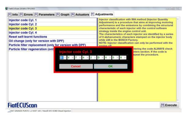
**Step 8:** Now we can enter the new injector code. We simply type **bv742dv5u** from the keyboard (or we can use the mouse and change each character).
