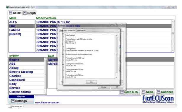
The "latency" values should be as low as possible. Usually it is below 10. The timer tests should match the reference values. A difference of up to 5% should not be a problem for correct operation.
