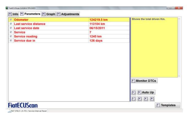
**Step 4:** Now we can go to the Adjustments screen and execute the service reset procedure.
