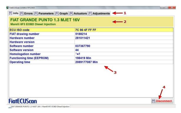
1. Using these buttons you can switch between the diagnostic windows of FiatECUScan. You can either click on the buttons or press the corresponding key on your keyboard:
