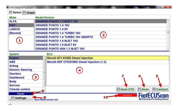
The main screen of FiatECUScan is divided into 4 parts. You can use the TAB button or the mouse to go from one part to another. You can also use the arrow keys to go up/down the lists.
