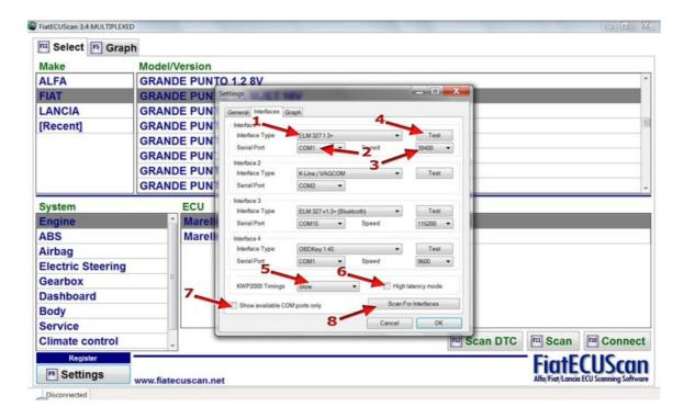
Here you can configure your interfaces. The program allows you to configure up to 4 interfaces. Each time when you try to connect to a car the program will check which of the configured interfaces is connected to the computer and try to use it. In most cases you can simply use the "Scan for Interfaces" functionality and it will automatically configure your interfaces. However, sometimes you need to configure the interfaces manually.
